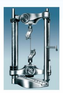
ATTACHMENT FOR TENSION TEST FOR WIRE ROPES.
