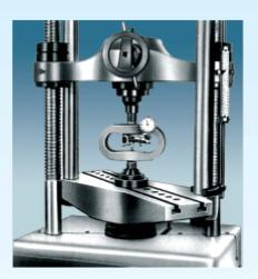
Calibration of Machine with providing Ring
