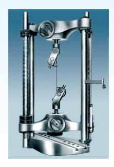
Attachment for Tension Test for Wire Ropes
